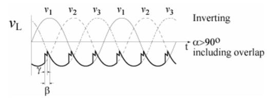
Anode voltage of fired thyristor > anode voltage on previously conducting thyristor over overlap interval
