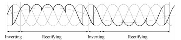
Each group operates alternately in rectifying and inverting modes
