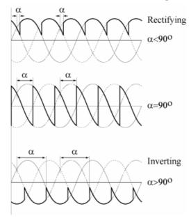
Thyristor may be fired when its anode voltage is higher than anode voltage of previously conducting thyristor, i.e. from α = 0° to α = 180°
