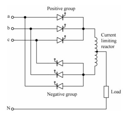
Cycloconverter require <u>complex control systems</u> – used for <u>high power</u> systems with variable frequency requirement <u>below frequency of an</u> <u>available AC supply</u>
