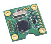
ZCT245AN-232 is a low cost 2-axis tilt sensor developed and produced by our company. Its measuring range is  $\pm$  45 degrees(range can be extended to 60 degrees). It can communicate with PC via RS232 half-duplex way. It has zero setting function and response frequency adjustment function as well as optional Baud rate
