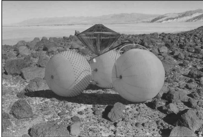
Figure 1-4: Inflatable Rover (Courtesy of NASA/JPL-Caltech)
